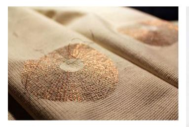
My industrial design graduation project investigated machine embroidery of electromagnetic coils, here implemented in a crystal AM radio receiver.
